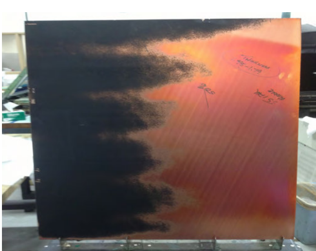
Figure 4: Plugged nozzles in developer chamber. Note uneven developing patterns on the test panel. (Source: RBP Chemical Technology)
