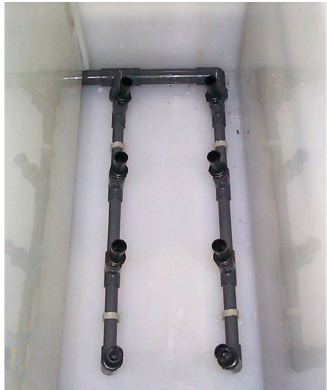
Figure 2: Actual photo of plating cell outfitted with bottom-up educators. (Source: RBP Chemical Technology)
