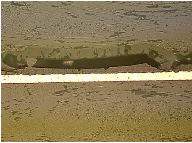
Figure 3: Delamination within the resin itself.
