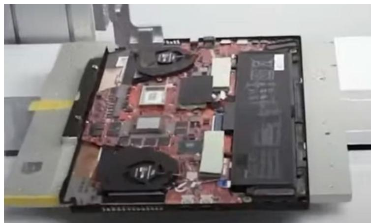
Figure 19: New generation of high-performance gaming notebook computers have solved the problem of cooling with new low-profile fans.
