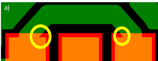
Figure 9: a) The original; b) The routing has changed a bit and the SMT corners have also been rounded. A possible problem solved.
