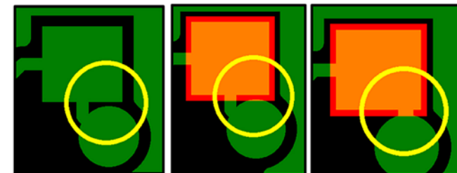
Figure 8: In the sample, the same net distance is below 45 \mu\text{m} .
