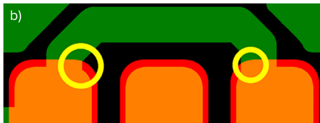
Figure 9: a) The original; b) The routing has changed a bit and the SMT corners have also been rounded. A possible problem solved.
