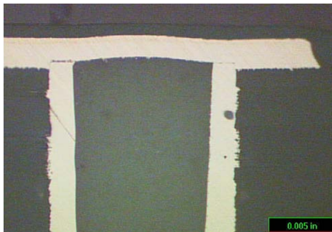
Figure 10: Excessive CTE leading to plated copper lifting from filled via.
