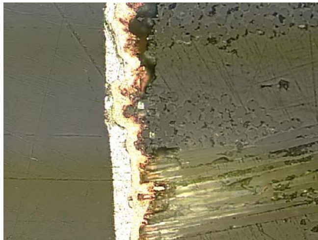
Figure 1: Rough hole wall due to poor drilling practice. Main cause—excessive in-feed rates of the drill tool.
