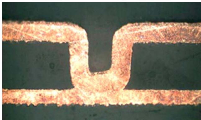
Figure 7: Example of conformal acid copper plating in a blind via.
