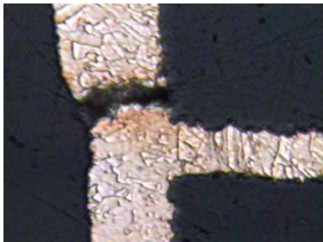
Figure 2: Barrel cracks in PTH subjected to thermal cycling. Note that the copper-to-inner-layer connections remain intact.
