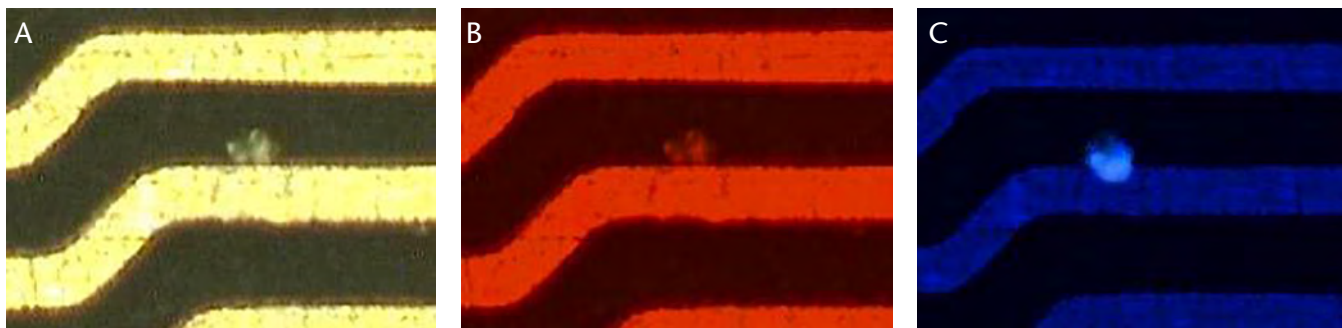
Figure 1: a) Microscopic image showing possible copper defect; b) using light source 1—still uncertain; c) light source 2—dust/pseudo-defect detected.
