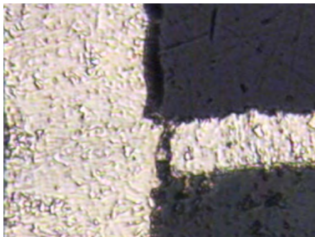
Figure 3: Interconnect defect (Source: IPC 9121).
